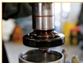
Remove the shock shaft from the shock body.
