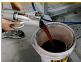
Have a bucket handy to dispose of all the used shock oil.
