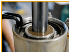
Be sure to completely discharge the nitrogen from the shock before going further. using the snapping pliers, remove the snap ring.
