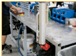
Be sure to secure the shock upside down in a good, strong table vise.
