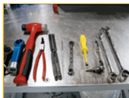
Valve tool, hammer, snapping pliers, cap tool, pick, ratchet wrench, nut driver, allen wrench, 3/4-inch open-end wrench, and 7/8-inch open-end wrench is all you need.
