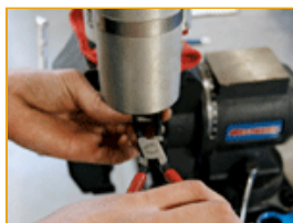
Use the snap-ring pliers to remove the snap ring on the other end of the reservoir can.
