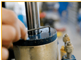
Use a 5/32-inch allen wrench to remove the set screw in the blue bearing cap.
